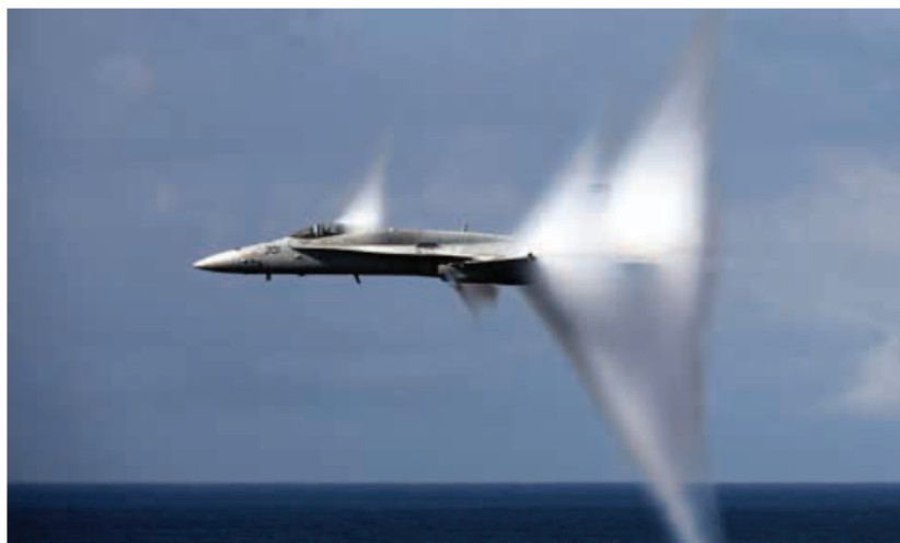
A supersonic jet traveling faster than the speed of sound. The vapor cone behind the jet is a cloud of condensed water that forms due to humid air entering a low-pressure region.
